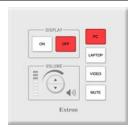
14. Press "Off "on button panel to shut down the system
